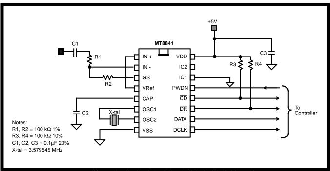
Figure 6 - Application Circuit (Single-Ended Input)
