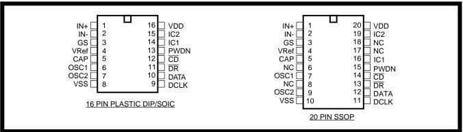
Figure 2 - Pin Connections
