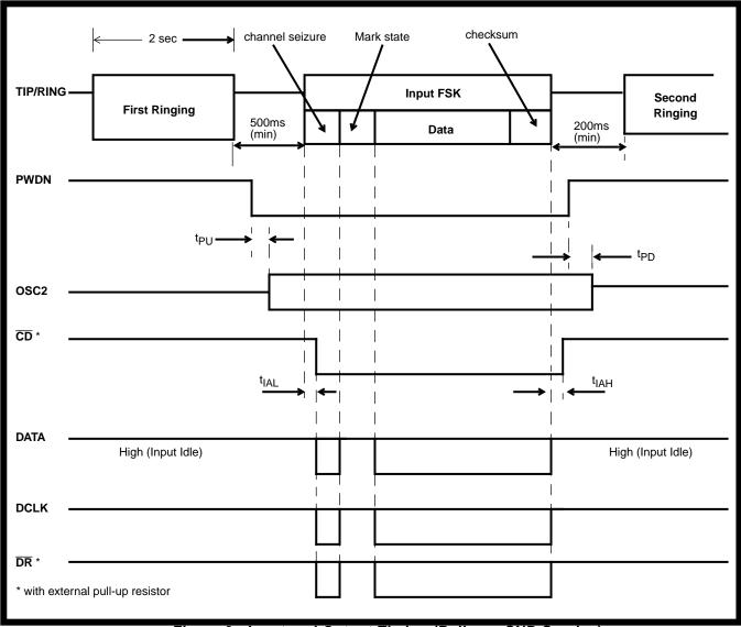
Figure 9 - Input and Output Timing (Bellcore CND Service)
