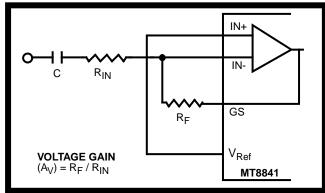
Figure 4 - Single-Ended Input Configuration
