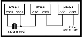
Figure 5 - Common Crystal Connection
