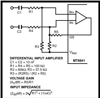
Figure 3 - Differential Input Configuration
