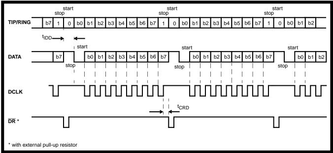
Figure 10 - Serial Data Interface Timing
